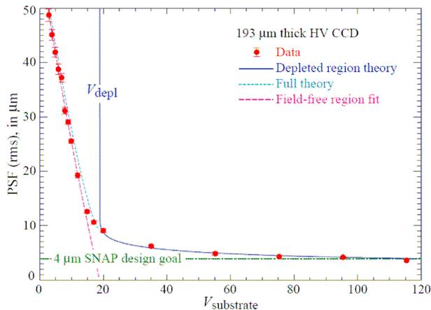
Figure 6. The measured rms diffusion as a function of the substrate bias voltage; the data are the red points, the magenta curve is the theoretical fit for operation below full depletion, the dark blue curve is the theoretical prediction for over-depleted operation, and the light blue curve is the convolution of both curves.
