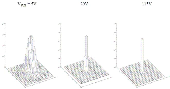
Figure 4. The spot image for three different substrate bias voltages. Full depletion is reached at 20 V.
