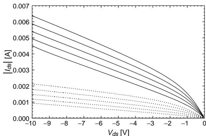
Fig. 9. Room temperature output characteristics of a 51/2 buried channel PMOSFET with 1.5  $\mu\text{m}$  gate to source/drain spacing (lower curves, dotted) compared to a self-aligned transistor (upper curves, solid). The substrate bias was 25V. The gate voltage was varied from 7.5 to 3.5V in 1V steps.
