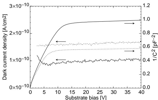
Fig. 5. Inverse square capacitance and reverse leakage current measured at room temperature on 2  $\text{mm}^2$  p-i-n diode test structures from CCD wafers. Data are shown for 200  $\mu\text{m}$  (dotted lines) and 275  $\mu\text{m}$  (solid lines) thick wafers.
