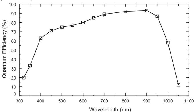
Fig. 6. Quantum efficiency measured on a 1980  $\times$  800, 15  $\mu\text{m}$  pixel back-illuminated, fully-depleted CCD. The measurement was performed at Lick Observatory and the operating temperature was  $-130^\circ\text{C}$ . The thickness was  $\approx 280 \mu\text{m}$ .
