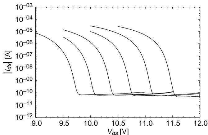
Fig. 8. Measured subthreshold characteristics of a 47/6 buried channel PMOSFET with  $1.5 \mu\text{m}$  gate to source/drain spacing. The substrate bias varied from 25V (rightmost curve) to 75V (leftmost curve) in 10V steps. The temperature was  $-128^\circ\text{C}$ , and the drain to source voltage was  $-1\text{V}$ .
