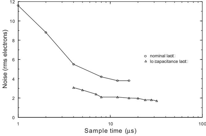
Fig. 13. Noise after double-correlated sampling versus sample time at  $-130^\circ\text{C}$  comparing 47/6 output transistors with varying size metal interconnect between the floating diffusion and output transistor.
