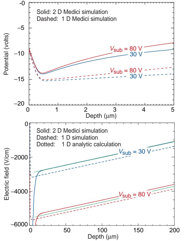
Fig. 18. Simulated potentials and electric fields versus depth for a CCD operated overdepleted. The dotted lines shown in the electric field plot were calculated from Equations A9 and A11 with  $V_J$  and  $y_N$  adjusted to give a good fit for the 30V case. The potential and field are plotted along the center line of the pixel.
