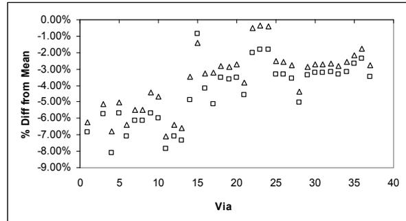
**Figure 16.** Flatfielding image for two colors. The diamonds show the via residuals after dividing a blue image by a red image, with both images taken at the same temperature. The squares show the via residuals after dividing a blue image by a red image but with the images taken at different temperatures ( $\Delta T \sim 10$  K).
