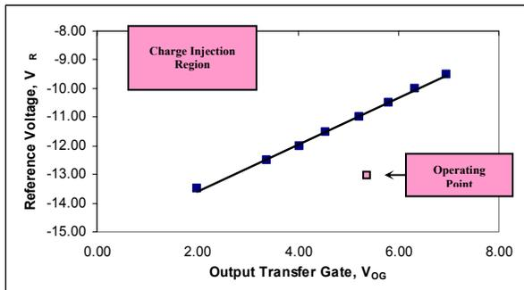
**Figure 7.** Output transfer gate transfer curve used to determine optimal output gate and reset drain voltages.
