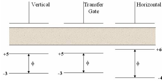
**Figure 9.** Standard clocking levels for LBNL designed high-resistivity CCDs.
