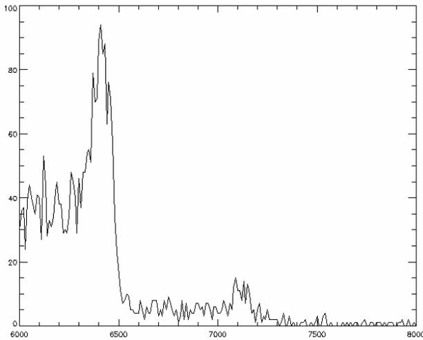
**Figure 19.** Histogram from an LBNL CCD illuminated with a Cd-109 x-ray source showing the energy captured in individual pixels. The  $K_{\alpha}$  and  $K_{\beta}$  peaks occur at 6400 ADU and 7150 ADU respectively.
