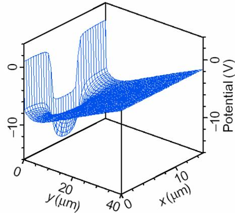
**Figure 2.** A two-dimensional simulation showing the potential in a fully-depleted LBNL CCD that directs the photo-generated carriers into the traditional potential wells formed by voltages on the frontside CCD gate electrodes.
