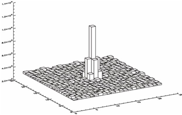
**Figure 17.** A sub-image from a 300  $\mu\text{m}$  thick, 15  $\mu\text{m}$  pixel pitch, LBNL CCD backside illuminated by a pinhole source with  $V_{\text{sub}} = 20$  V.
