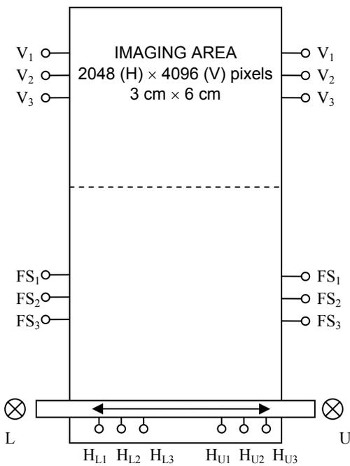
**Figure 3.** Schematic of the 2048 × 4096-pixel LBNL CCD. V and FS indicate the vertical and framestore parallel clocks. The upper and lower readout stages are labeled U and L respectively. The serial register has independent upper and lower horizontal clock lines.
