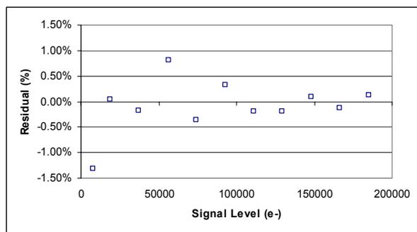
**Figure 14.** Residual difference of linearity transfer data from a least-squares fit to the measurements.
