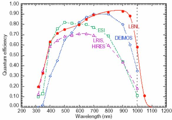
**Figure 11.** Measured quantum efficiencies comparing a 300 mm thick, fully depleted LBNL CCD versus CCDs in use at the Keck Telescope. The ESI and DEIMOS CCD's were fabricated at MIT Lincoln Laboratory [3], and the HIRES/LRIS CCD's were fabricated at Scientific Imaging Technologies.
