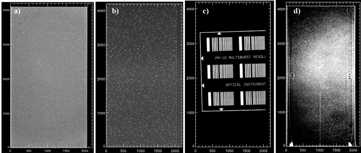
**Figure 6.** Images taken on the MSL fabricated 2k×4k device selected for further testing: **a)** a bias frame, **b)** Cd-109 X-Ray image, **c)** a resolution bar target image, and **d)** 10,000  $e^-$  level green flat field image ( $650 \pm 21$  nm). All images are set to maximum stretch.
