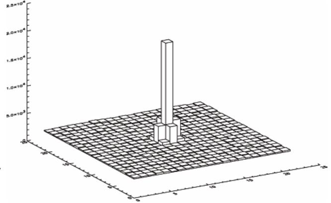
**Figure 18.** A sub-image from a 300  $\mu\text{m}$  thick, 15  $\mu\text{m}$  pixel pitch, LBNL CCD backside illuminated by a pinhole source with  $V_{\text{sub}} = 60$  V.
