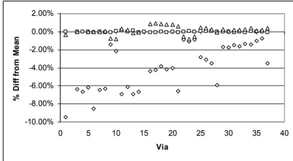
**Figure 15.** Flatfielding data for one color, blue. The diamonds show the initial levels of the vias prior to flatfielding (see Figures 9 and 10). The squares show the via levels after division of an image through a blue filter by another blue image at the same temperature. The triangles show the levels of the vias after division by a blue image at a different temperature ( $\Delta T \sim 10$  K).
