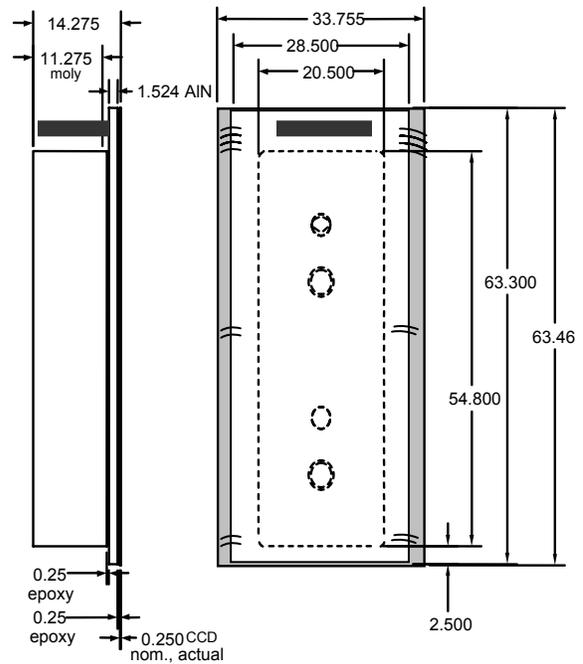
**Figure 4.** Four-side buttable package design for a 2k×4k device (units in mm). The primary parts of the package are the CCD, a printed AIN substrate, a Moly foot, an electrical connector soldered on the AIN substrate, and wirebonds that connect the CCD to the AIN substrate.
