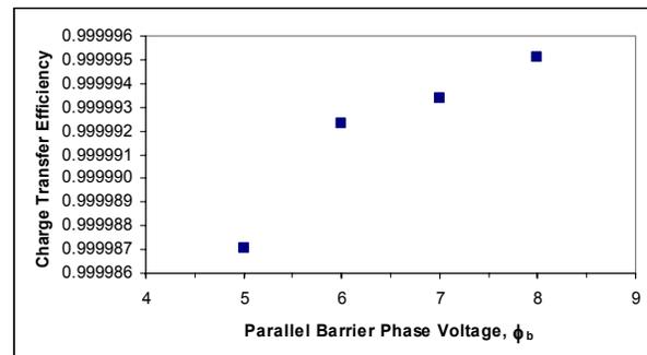
**Figure 8.** Parallel charge transfer efficiency measured as a function of the barrier voltage via the EPER method.
