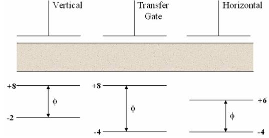
**Figure 10.** Optimized clocking levels for a MSL-fabricated 2kx4k high-resistivity LBNL CCD.
