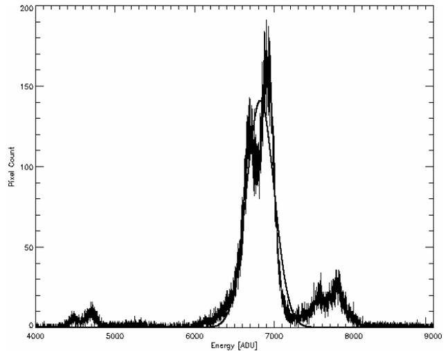
**Figure 20.** Histogram from an LBNL CCD illuminated with a Cd-109 x-ray source showing the energy captured in a  $3 \times 3$  square of pixels. The  $K_{\alpha}$  and  $K_{\beta}$  peaks occur at 6828 ADU and 7750 ADU respectively.
