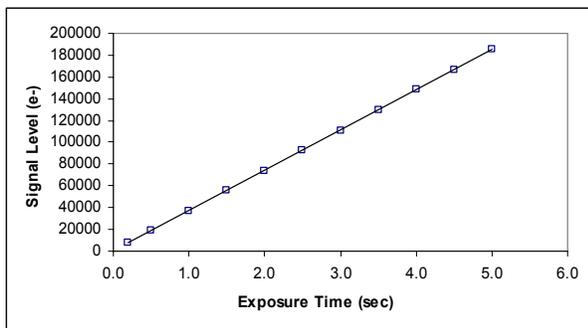
**Figure 13.** Linearity transfer curve showing the signal versus exposure time for a pinhole illumination.
