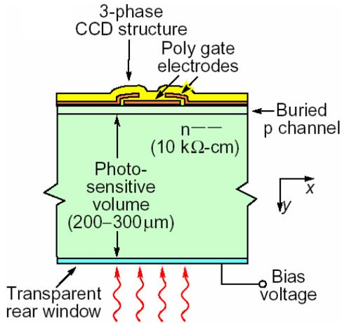
**Figure 1.** Cross section of the LBNL fully depleted CCD. A conventional buried channel CCD is fabricated on a high-resistivity silicon substrate. A bias voltage applied to the backside electrode results in full depletion.
